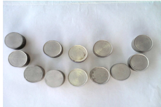
Figure 11. Sintered Specimen for Various Sample Pieces (Top Orientation).
