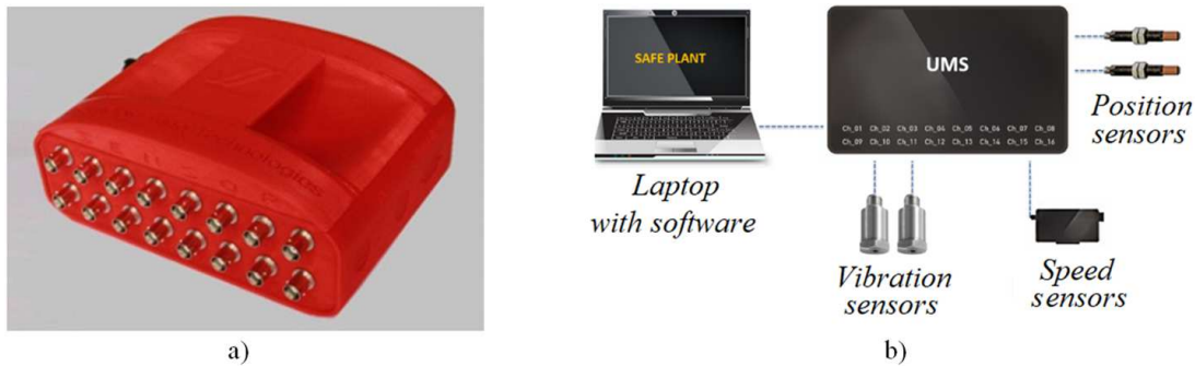
Figure 5. Measuring unit of the universal multichannel measuring system UMS-16 (a), schematic diagram of the UMS-16 complex in conjunction with the SAFE PLANT software (b).
