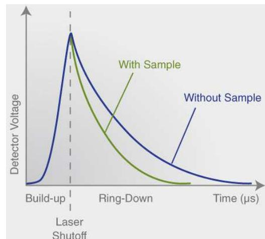
Figure 4. Light intensity as a function of time in a CRDS system with and without a sample having resonant absorbance. This demonstrates how optical loss (or absorption by the trace gas) is rendered into a time measurement [15].
