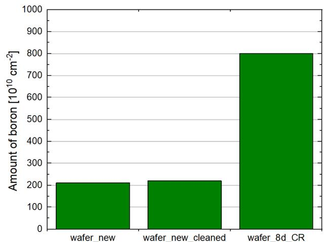
**Figure 16.** Amount of boron on monitoring wafers: new, cleaned and 8 days in cleanroom.
