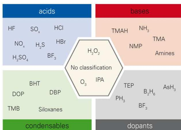
Figure 1. Classification of critical contaminations by ITRS [14].
