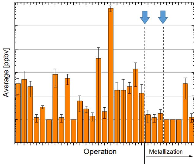
**Figure 7.** Concentration levels of AMC-2 contamination along the supply chain of one power technology. The blue arrows indicate the existing FOUF cleaning steps within the process flow.
