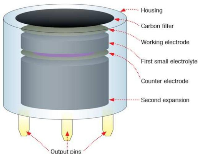
Figure 5. Schematic illustration of electrochemical conductivity cell [16].
