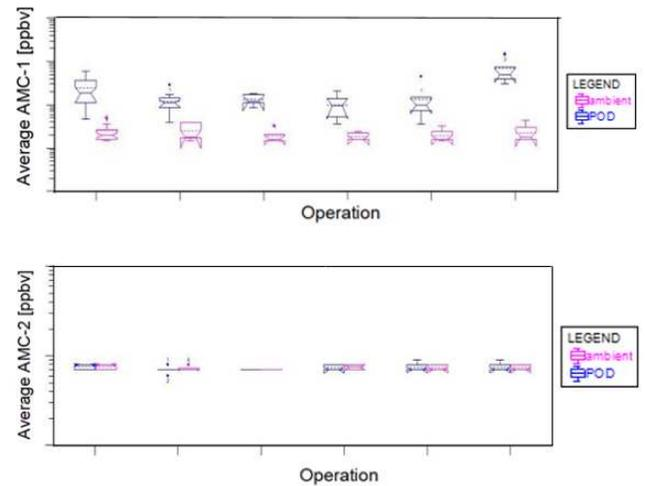
Figure 14. Concentration levels of contaminations out of AMC group 1 and 2 at dedicated work steps of the JFET process flow.
