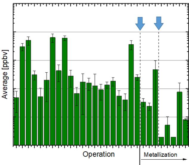
**Figure 8.** Concentration levels of AMC-1 contamination along the supply chain of one power technology. The blue arrows indicate the existing FOUF cleaning steps within the process flow.
