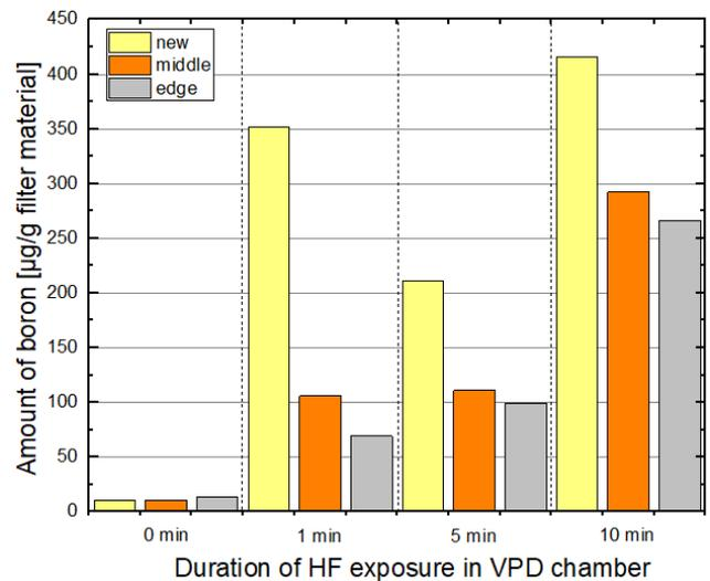
**Figure 18.** Amount of boron release from an old and new filter after different duration times in a defined HF atmosphere.
